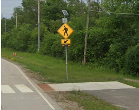
Rectangular Rapid Flashing Beacon
