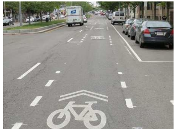
Priority shared-lane markings include additional striping to further establish the route as a bikeways. Image courtesy of Boston.com
