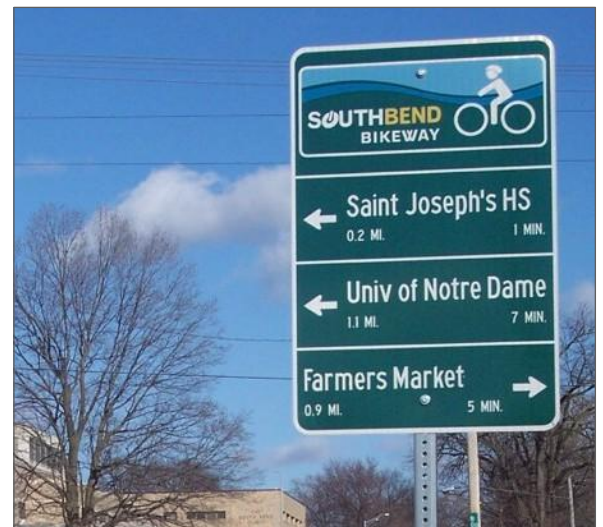
Wayfinding signs should include clear destination, direction and distance information (in both time and miles). Image courtesy of bicyclemichiana.org .
