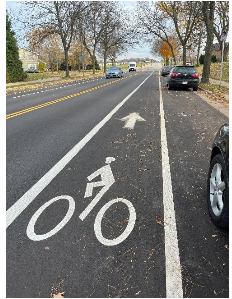
A conventional bicycle lane in Milwaukee, WI with striping and pavement marking
